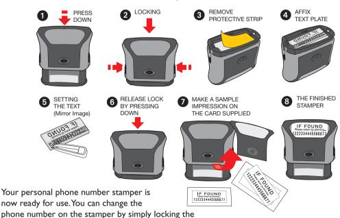
stamper as shown in the diagram, removing your old number and inserting your new number.
